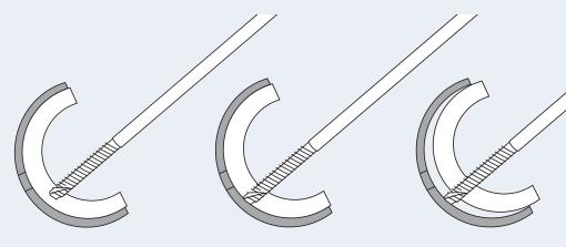
When the flat-ended drill end reaches the metal of the acetabular cup, continue drilling and the liner will become engaged in the drill flutes and back off for removal.
